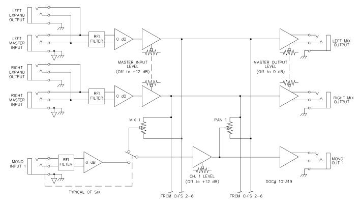
Figure 1. SM 26 Complete Block Diagram
