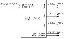
Figure 10. Four Channel Stereo Splitter
