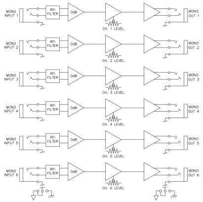
Figure 4. 6 In/6 Out Buffer Amplifier
