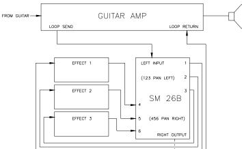
Figure 13. Mono Guitar Effects Splitter/Mixer
